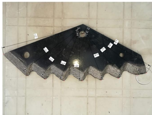
Fig. 1. Worn-out knife of the feed mixer Fig. 2. Scheme of measuring the knife geometry
