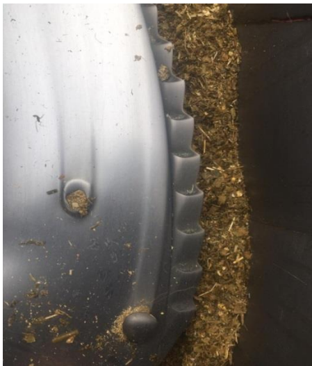
Fig. 1. Worn-out knife of the feed mixer Fig. 2. Scheme of measuring the knife geometry
