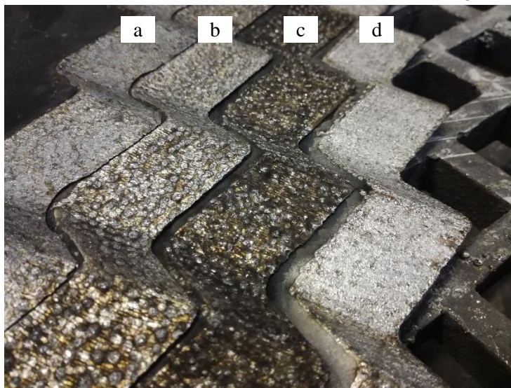
Fig. 4. Knives coated with different materials: a – T15K6 coating; b – P6M5 coating; c – T-590; d – VK8
